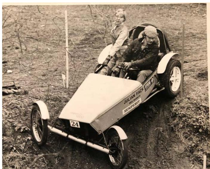
*Julian & Meg in Impunity 2, late-1970s. Note the raised tube behind the seat to bring it back inside the regulations. Like Impunity 1, the car featured the fabulous low seat until it was banned. Note also the very low bonnet line which meant the driver could see the bottom of both front wheels - important in the days of tight trials.*
