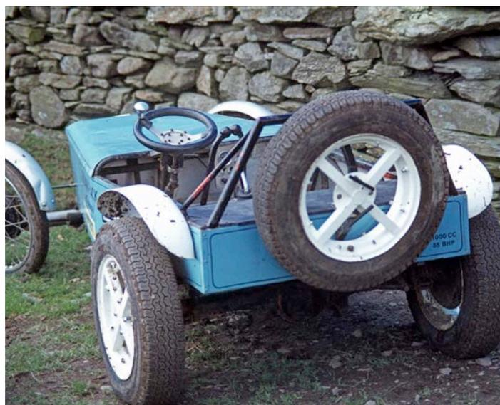
*Impunity 2 at a trial in Cumbria, 1977. Clearly visible is the low back which was subsequently banned. Note also the sticker proclaiming the engine to be 1000cc & 55bhp! It was upgraded to a 1200cc Imp the following year, after which it was extraordinarily successful for a couple of years.*
